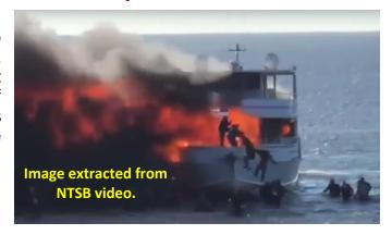
The fire was intense, fast moving and ultimately burned the vessel to the waterline. Investigators determined a number of causal factors that contributed to ignite and intensify the fire. This included a lack of company guidance regarding engine high-temperature alarms, lack of fire detection in unmanned spaces with exhaust tubing, insufficient preventive maintenance, insufficient crew training and documentation, and inappropriate material and design of the fuel tank level-indicator system.
